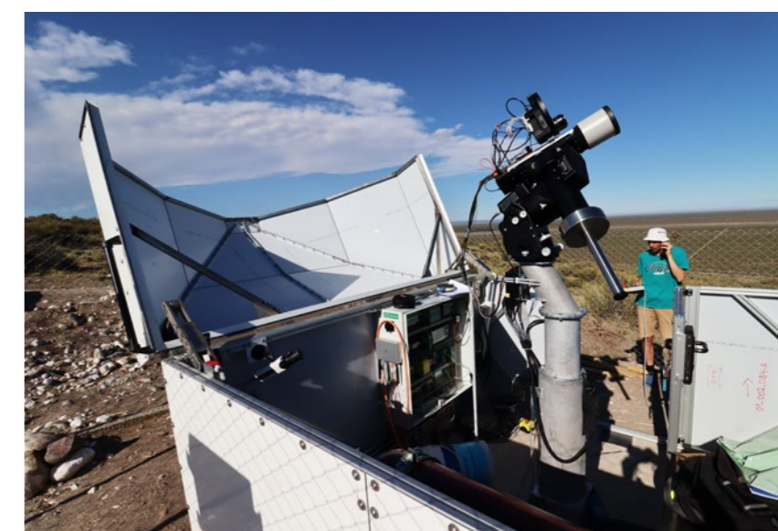
► AUGER-CZ – Telescope FRAM used to monitor atmospheric conditions at Pierre Auger Observatory in Argentina which detects the highest energy cosmic rays coming from the Universe
